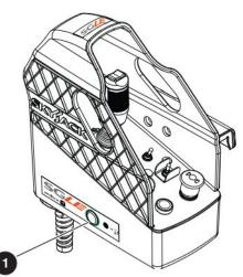
**SGLE:** This push-button energizes the lift function. Hold the button down together with the function-enable switch to raise the platform with the lift function.
