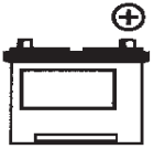
Positive Battery Terminal
