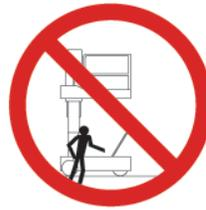
**DO NOT** access the hydraulic/electrical compartment while the platform is raised.
