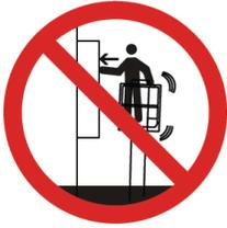
**DO NOT** exceed the maximum side force shown on the capacity label when the platform is elevated (refer to [Section 7.4](#)).
