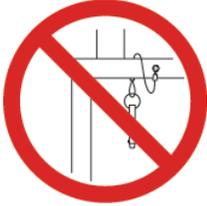
**DO NOT** use the MEWP without guardrails, lock pins, and the entry gate in place.
