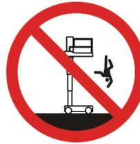
Prevent falls from the platform. Always keep a firm footing on the platform floor when working on it. Do not climb on the toe-board, mid-rail, or top-rail. Do not use planks, ladders, or any other devices on the platform to get more height or reach.
