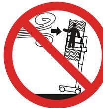
**DO NOT** increase the surface area of the platform or carry large surface area items when exposed to wind. Increasing the area exposed to the wind will decrease the MEWP stability.
