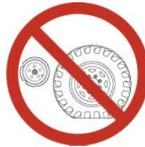
**DO NOT** use the MEWP when the wheels or tires are damaged. Make sure the wheel nuts and cotter pins are in place (refer to [Section 4.2-6](#)).
