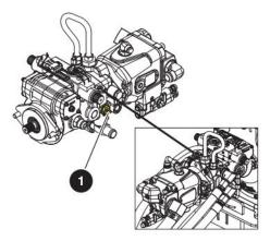
Figure 28 Drive Bypass Valve
