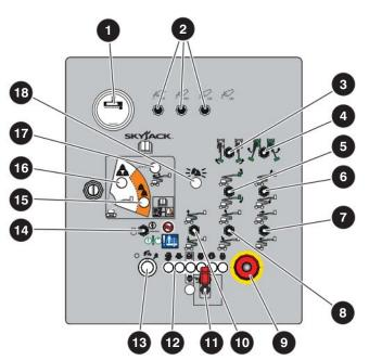
Figure 07 Base control console
