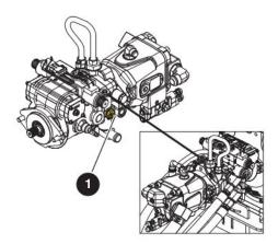
Figure 29 Drive bypass valve
