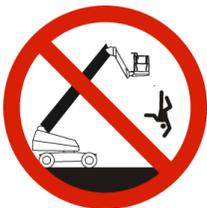
**AVOID** falling. Stay within the boundaries of the guardrails. Maintain firm footing on the platform floor at all times while working thereon.
