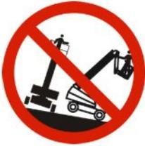
**DO NOT** ascend or descend a grade steeper than 45% (4WD). Boom elevated driving must only be done on firm, level surfaces.
