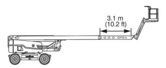
Figure 13 Fly boom extension into low capacity zone
