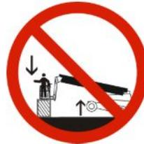
**DO NOT** use boom to push, pull other objects or to lift the chassis.
