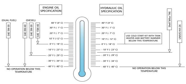
Figure 25 Cold weather operation chart
