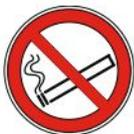
**Explosion hazard. Keep flames and sparks away. Do not smoke near batteries. Battery acid releases explosive gas while charging. Charge batteries in a well-ventilated area.**
