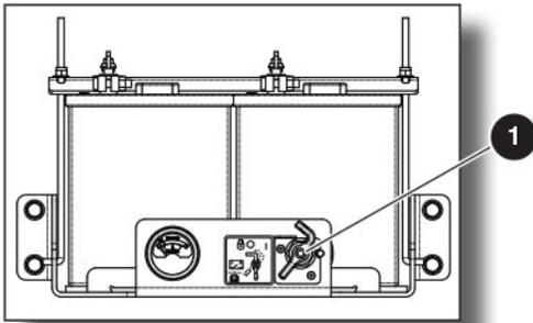
Figure 06 Main power disconnect switch
