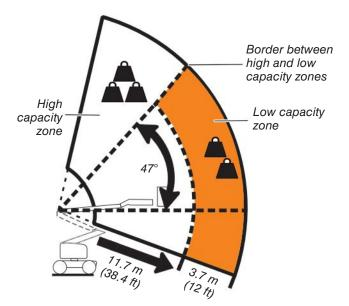
Figure 12 High and low capacity zones
