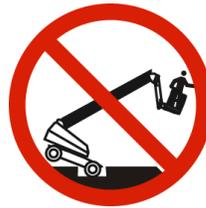
**DO NOT** drive elevated near depressions or holes of any type, loading docks, debris, drop-offs and surfaces that may affect the stability of the MEWP.
