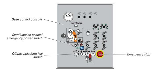
4.3-4 Testing start/function enable/ emergency power switch and all boom and platform functions
