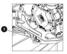
Figure 21 Battery warmer/Hydraulic oil heater cord
