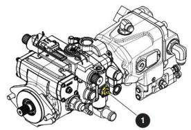
Figure 16 Drive bypass valve
