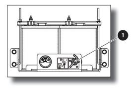
Figure 06 Main power disconnect switch
