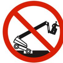
**If operation in areas with holes or drop-offs is absolutely necessary,** elevated driving shall not be allowed. Position the MEWP horizontally only with the platform fully lowered. After ensuring that all 4 wheels or outriggers (if equipped) have contact with a firm, level surface, the MEWP can be elevated. After elevation, the drive function must not be activated.
