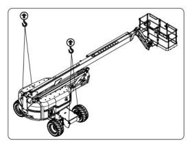
Figure 35 Lifting points
