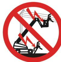
**MAINTAIN** a minimum safe approach distance from sources of high-voltage power.
