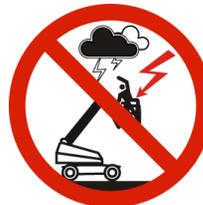
**DO NOT** operate the MEWP during lightning or storms. Take into account the effects of weather (e.g., wind, rain and snow) on the safe operation of the MEWP.
