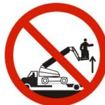
**DO NOT** raise the MEWP while it is on a truck, forklift or other device or vehicle.
