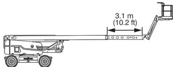
Figure 13 Fly boom extension into low capacity zone
