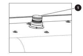
Figure 19 Flashing amber light
