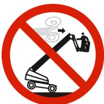
**DO NOT** raise the MEWP or operate elevated in windy or gusty conditions that exceed the limits specified in [Section 7.7](#).
