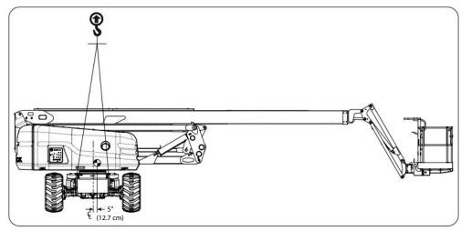
Figure 36 Center of gravity
