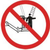
**DO NOT** operate an MEWP that has ladders, scaffolding or other devices mounted on it to increase its size or work height. It is prohibited.
