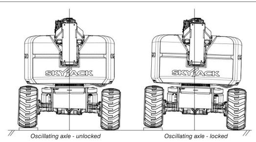
4.3-26 Testing oscillating axles
