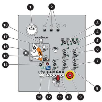
Figure 08 Base control console
