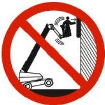
**DO NOT** exert horizontal (manual) force on MEWP that exceeds the limits specified in [Section 7.7](#).
