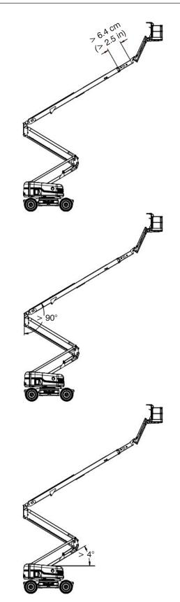
Figure 11 Elevated travel position (any of the boom positions shown)
